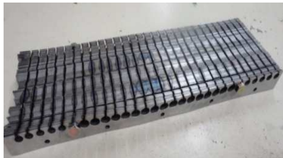
Figure 6: Laminated Silicon Steel (STATOR)
